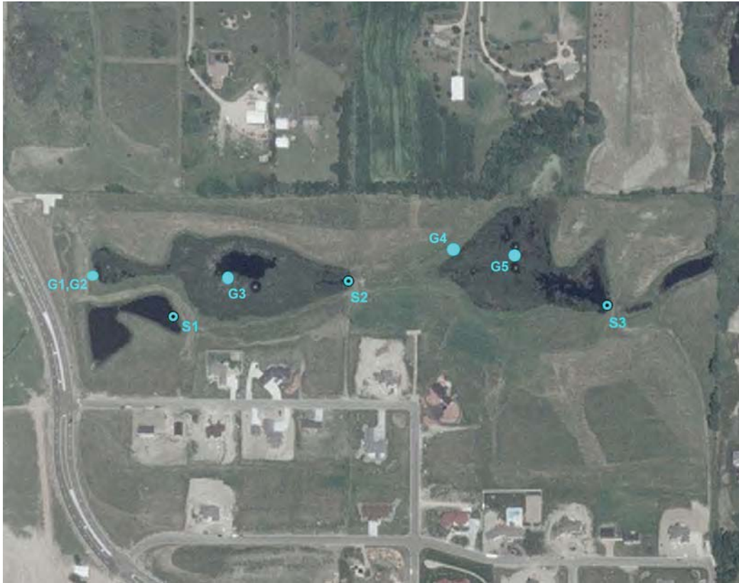
Figure 9. Aerial photo of the Prior Lake wetland system with the surface water temperature (S1 – S3) and groundwater temperature (G1-G5) measurement stations. Groundwater and surface water flows from left to right.
