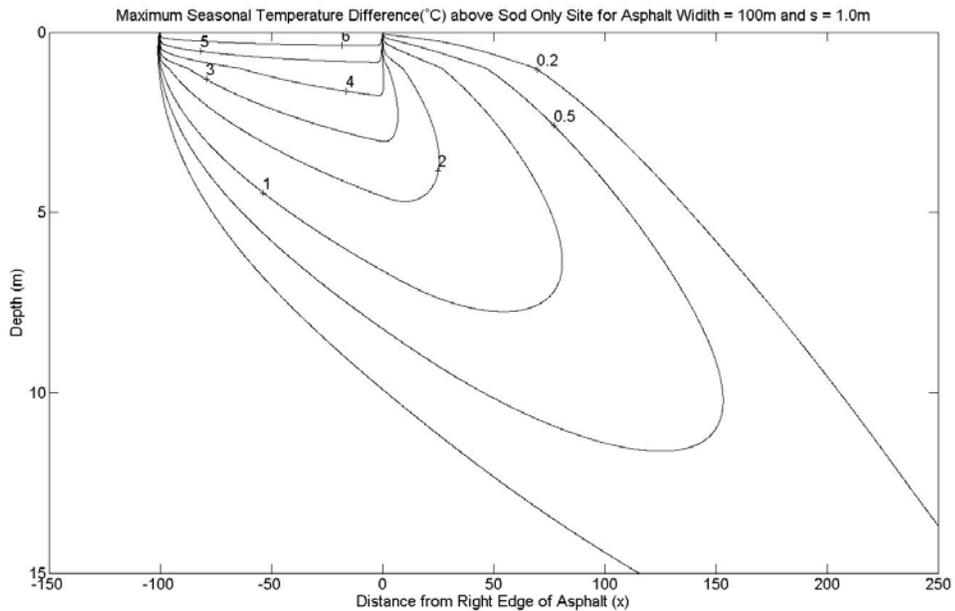
Figure 3.7 Excess temperature plume for a composite grass-asphalt-grass surface cite. The excess temperature ( $^{\circ}\text{C}$ ) is the degrees above the temperature of a grass only site at the same location/depth. Parameter values are:  $W = 100\text{m}$ ,
