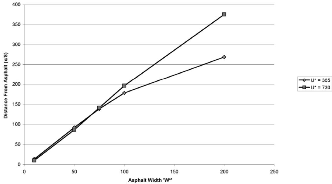
Figure 5.8 Critical normalized distance from pavement ( $x^*$ ) vs. normalized pavement width ( $W^*$ ) (corresponding to Figures 5.3 and 5.5).
