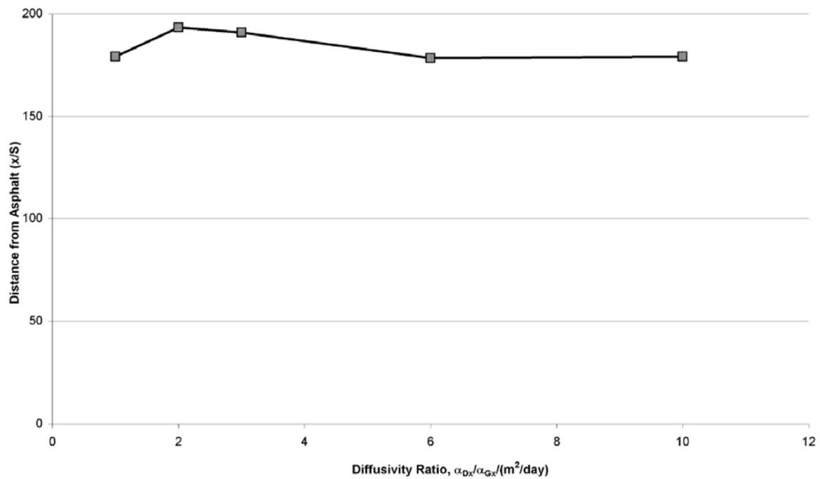
Figure 5.9 Critical distance from pavement ( $x^*$ ) vs. diffusivity ratio in  $x$ -direction ( $\alpha_{Dx}/\alpha_{Gx}$ ) (corresponding to Figure 5.4).
