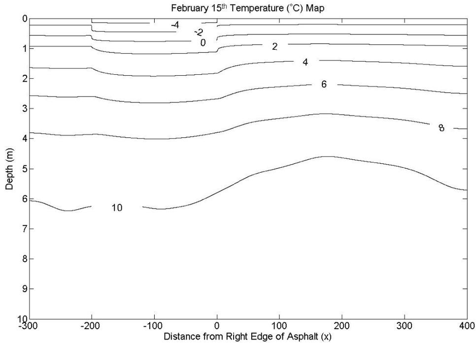
Figure 3.3a Instantaneous temperature field given by isotherms in the unsaturated zone and groundwater domain for February 15. Asphalt extends from  $x = -200m$  to  $0m$ . Groundwater is flowing in the  $x$ -direction. Parameter values are:  $W = 200m$ ,  $S = 1.0m$ ,  $h = 20m$ ,  $u = 1.0m/day$ ,  $\alpha_{Dx} = \alpha_{Dy} = 0.07m^2/day$ ,  $\alpha_{Gx} = 0.42m^2/day$ , and  $\alpha_{Gy} = 0.14m^2/day$ .
