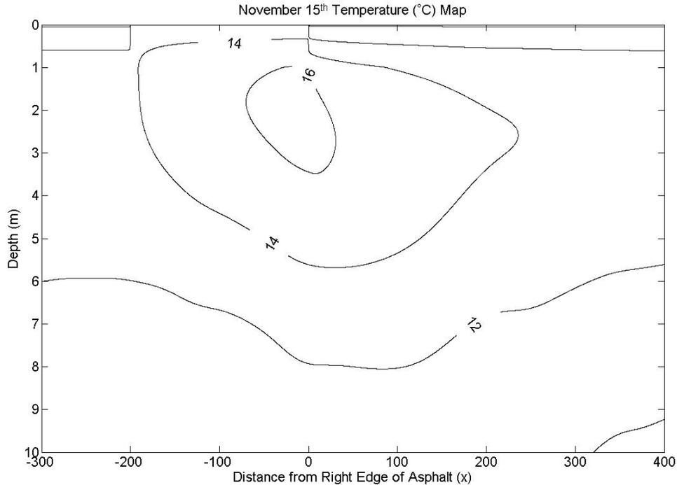
Figure 3.3d Instantaneous temperature field given by isotherms in the unsaturated zone and groundwater domain for November 15. Asphalt extends from  $x = -200m$  to  $0m$ . Groundwater is flowing in the  $x$ -direction. Parameter values are:  $W = 200m$ ,  $S = 1.0m$ ,  $h = 20m$ ,  $u = 1.0m/day$ ,  $\alpha_{Dx} = \alpha_{Dy} = 0.07m^2/day$ ,  $\alpha_{Gx} = 0.42m^2/day$ , and  $\alpha_{Gy} = 0.14m^2/day$ .
