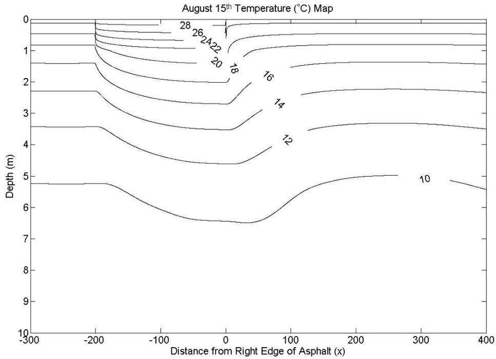
Figure 3.3c Instantaneous temperature field given by isotherms in the unsaturated zone and groundwater domain for August 15. Asphalt extends from  $x = -200m$  to  $0m$ . Groundwater is flowing in the  $x$ -direction. Parameter values are:  $W = 200m$ ,  $S = 1.0m$ ,  $h = 20m$ ,  $u = 1.0m/day$ ,  $\alpha_{Dx} = \alpha_{Dy} = 0.07m^2/day$ ,  $\alpha_{Gx} = 0.42m^2/day$ , and  $\alpha_{Gy} = 0.14m^2/day$ .
