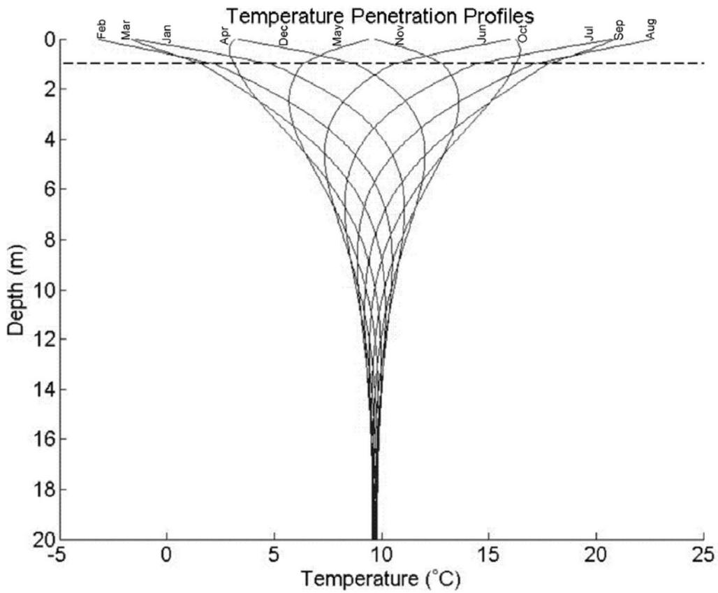
Figure 3.1 Temperature penetration profiles under a grass surface ( $S = 1.0\text{m}$ ,  $h = 20\text{m}$ ,  $\alpha_{Dx} = \alpha_{Dy} = 0.07\text{m}^2/\text{day}$ ,  $\alpha_{Gx} = 0.42\text{m}^2/\text{day}$ ,  $\alpha_{Gy} = 0.14\text{m}^2/\text{day}$ ,  $T_{m,g} = 9.7^\circ\text{C}$ , and  $\Delta T_g = 13.0^\circ\text{C}$ )
