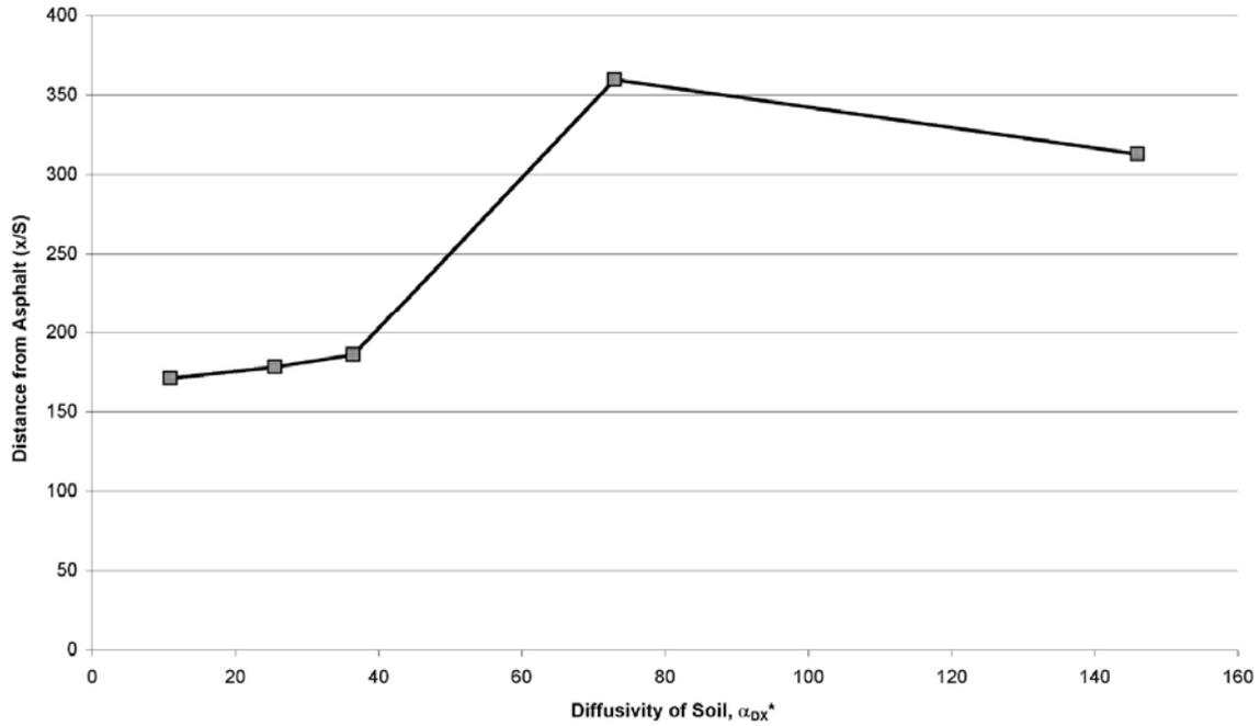
Figure 5.6 Critical normalized distance from pavement ( $x^*$ ) vs. normalized thermal diffusivity in the dry soil ( $\alpha_{Dz}^*$ ) (corresponding to Figure 5.1)
