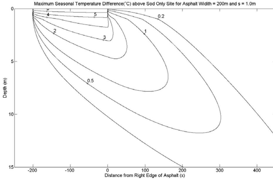
Figure 3.5 Excess temperature plume for a composite grass-asphalt-grass surface cite. The excess temperature ( $^{\circ}C$ ) is the increment above the temperature of a grass only site at the same location/depth. ( $W = 200m$ ,  $s = 1.0m$ ,  $h = 20m$ ,  $u = 2.0m/day$ ,  $\alpha_{Dx} = \alpha_{Dy} = 0.07m^2/day$ ,  $\alpha_{Gx} = 0.42m^2/day$ , and  $\alpha_{Gy} = 0.14m^2/day$ )
