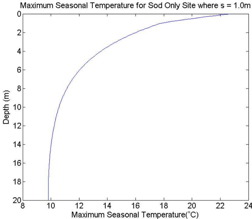
Figure 3.2 Maximum annual temperatures ( $^{\circ}\text{C}$ ) under a grass surface ( $S = 1.0\text{m}$ ,  $h = 20\text{m}$ ,  $\alpha_{Dx} = \alpha_{Dy} = 0.07\text{m}^2/\text{day}$ ,  $\alpha_{Gx} = 0.42\text{m}^2/\text{day}$ ,  $\alpha_{Gy} = 0.14\text{m}^2/\text{day}$ ,  $T_{m,g} = 9.7^{\circ}\text{C}$ , and  $\Delta T_g = 13.0^{\circ}\text{C}$ ).
