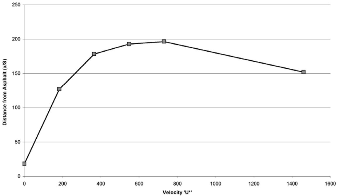
Figure 5.7 Critical normalized distance from pavement ( $x^*$ ) vs. normalized groundwater flow velocity ( $U^*$ ) (corresponding to Figure 5.2).
