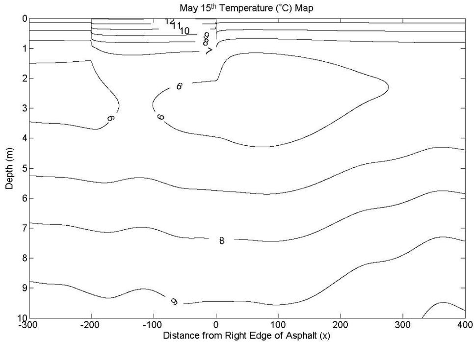
Figure 3.3b Instantaneous temperature field given by isotherms in the unsaturated zone and groundwater domain for May 15. Asphalt extends from  $x = -200m$  to  $0m$ . Groundwater is flowing in the  $x$ -direction. Parameter values are:  $W = 200m$ ,  $S = 1.0m$ ,  $h = 20m$ ,  $u = 1.0m/day$ ,  $\alpha_{Dx} = \alpha_{Dy} = 0.07m^2/day$ ,  $\alpha_{Gx} = 0.42m^2/day$ , and  $\alpha_{Gy} = 0.14m^2/day$ .
